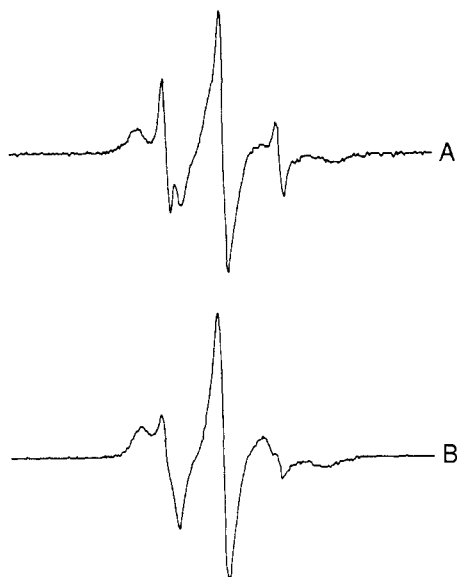
Figure 11. EPR spectrum (A) of labeled cell walls treated with 2 N KOH and fully hydrated to 0.85 g of bound \text{H}_2\text{O} /g of cell walls. EPR spectrum (B) of a \text{Ca}^{2+} -doped sample A (0.88 \text{Ca}^{2+} per binding site) and hydrated to a level of 1.1 g of \text{H}_2\text{O} /g of solid.
